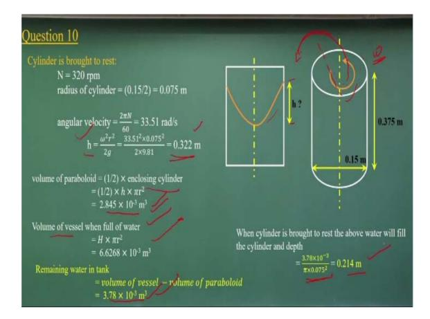
Now the first what is that if n is rotations per minute and you compute the radius, Cylinder is brought to rest:
